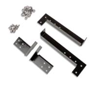
The PulseTech Bracket Kit is an accessory for the 24VPSC-10W Solar Pulse Charger (735X724), NSN 6130-01-688-4857. This bracket kit is used for quick and secure mounting of the charger to LMTV vehicles that have plastic molded snorkels. It is designed with two shorter brackets at the front and longer brackets at the back to allow for an angled solar panel mount for maximum sun exposure. One year limited warranty.
