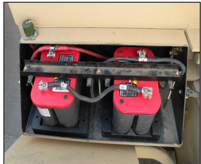
Optima Red Top 34 with 6T Adapter Plate shown Battery NSN 6140-01-378-8232 6T Adapter Plate NSN 6160-01-453-0858
