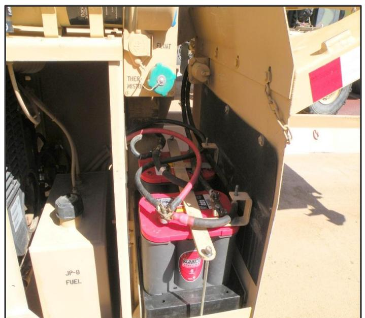
**Optima Red Tops model 34 with 6T Adapter Plate
